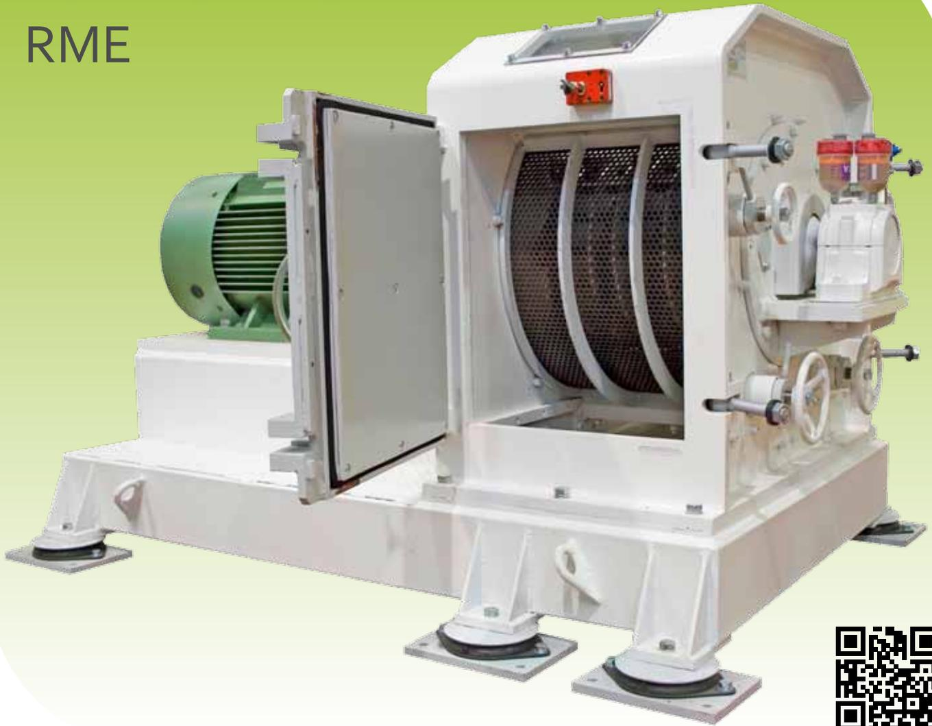
The RME hammermill is derived from the RM range. It is adapted to meet reliability criteria required by industries requiring a very high mechanical and wearing strength to face high impact loads (knackery, paper blocks, cakes, cassava roots, etc...)
