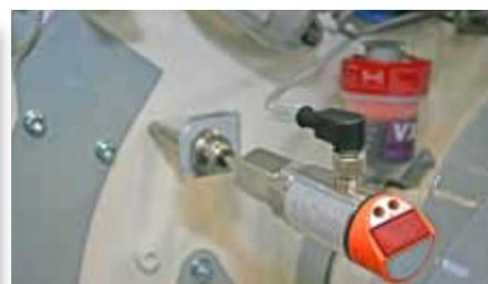
Temperature gauge on grinding chamber
