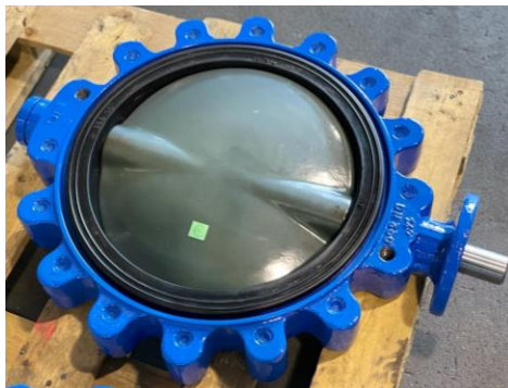
DN350 Halar coated disc
