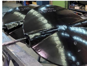
Final epoxy coating
